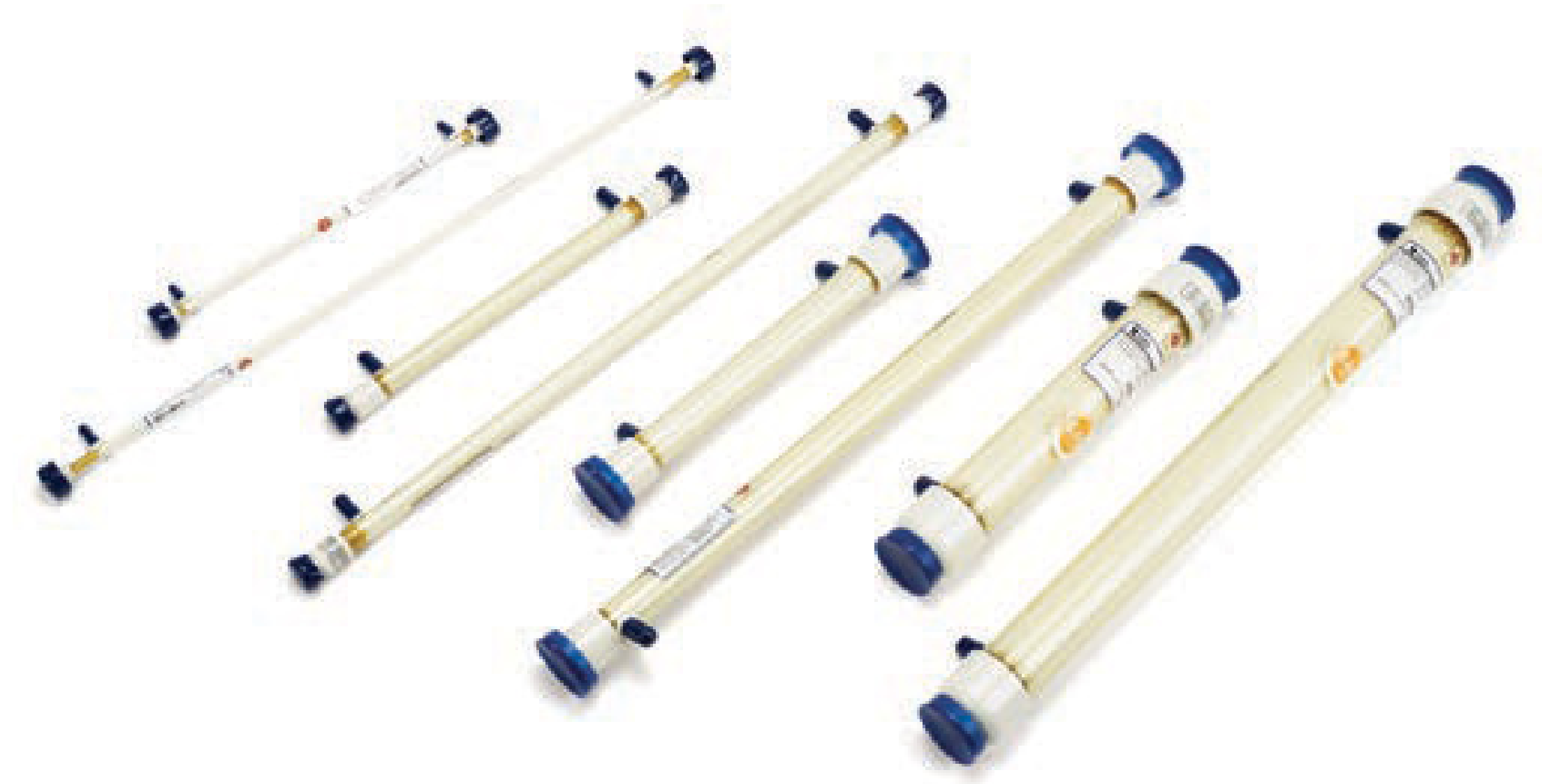
Fig 6. Cytiva's 750 C hollow-fiber filter, with a M_r 750 000 nominal molecular weight cutoff (NMWC), is designed for use in virus-purification workflows. It effectively removes ovalbumin and other proteins in allantoic fluid from egg-based virus production as well as host-cell-derived impurities from production in cells. When compared with a 500 C hollow-fiber filter — with the same 0.5 mm lumen diameter but a M_r 500 000 NMWC — in a concentration and diafiltration process, the more open structure of the 750 C filter gave a 1.5–2.0 orders of magnitude higher host cell DNA (hcDNA) removal at similar host cell protein (HCP) removal and virus yield (6).
