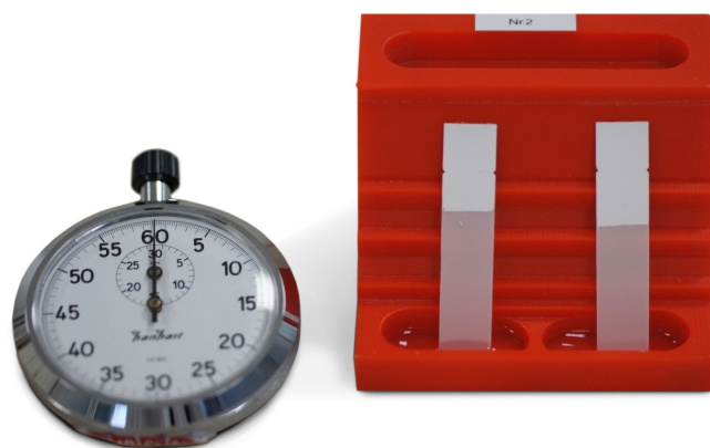
Fig 1. Basic set-up of membrane capillary flow time measurement. Strip width is 1 cm, strip length 4.5 cm, with triangular marks at 4 cm strip length. The time the liquid (water) needs to reach these marks is taken and documented. Water volume is 100 \mu L.
