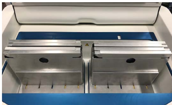
Fig 1. A view of the cryochamber within the VIA Freeze Quad unit with sample plates loaded with 8 × 70 mL cryobags held in metal cassettes.
