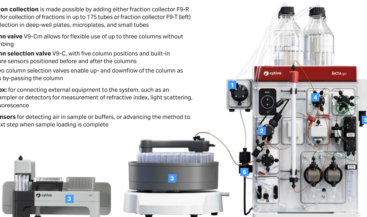
Fig 4. Optional components can be added in the two empty positions in the system chassis or mounted on rails to expand the capability of the ÄKTA go™ system. As many as six options can be added at the same time. One fraction collector can be added; either F9-T or F9-R.
