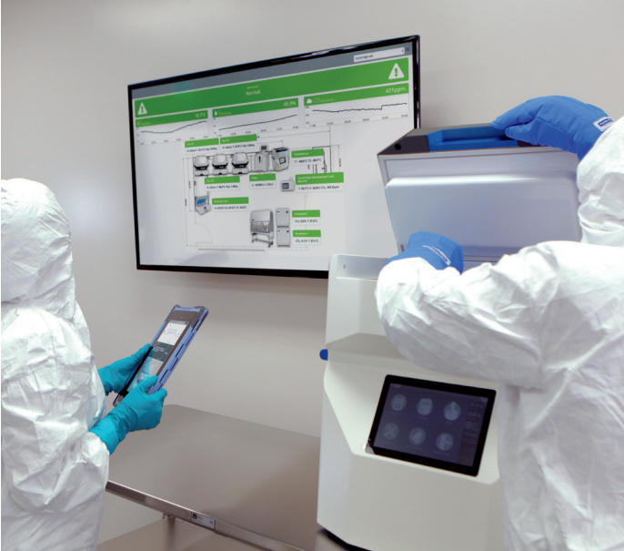
Fig 3. A Chronicle dashboard shows the live status of every instrument in the cleanroom.
