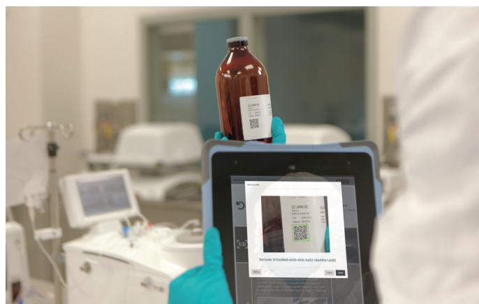
Fig 2. An operator scans a reagent label to identify lot number and expiration date.
