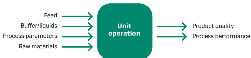
Fig 5. Input/output diagram showing factors that could affect product quality and process performance.
