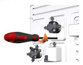
4 Remove the module or module panel and disconnect the cable at the back.
