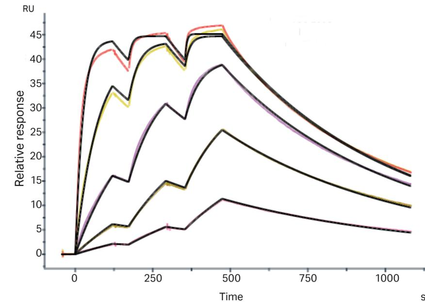
The model does not fit the data for the highest analyte concentrations.
