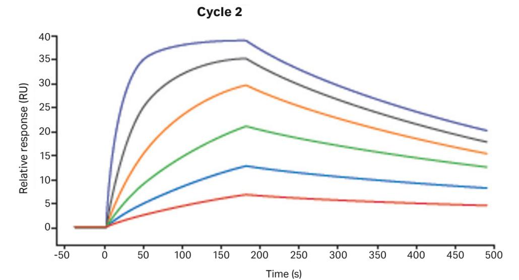
**Note:** Parallel kinetics is run in a single cycle for each analyte concentration series, but should not be confused with single-cycle kinetics. The term single-cycle kinetics is reserved for the experimental format where analyte concentrations are injected sequentially in the same flow channel.
