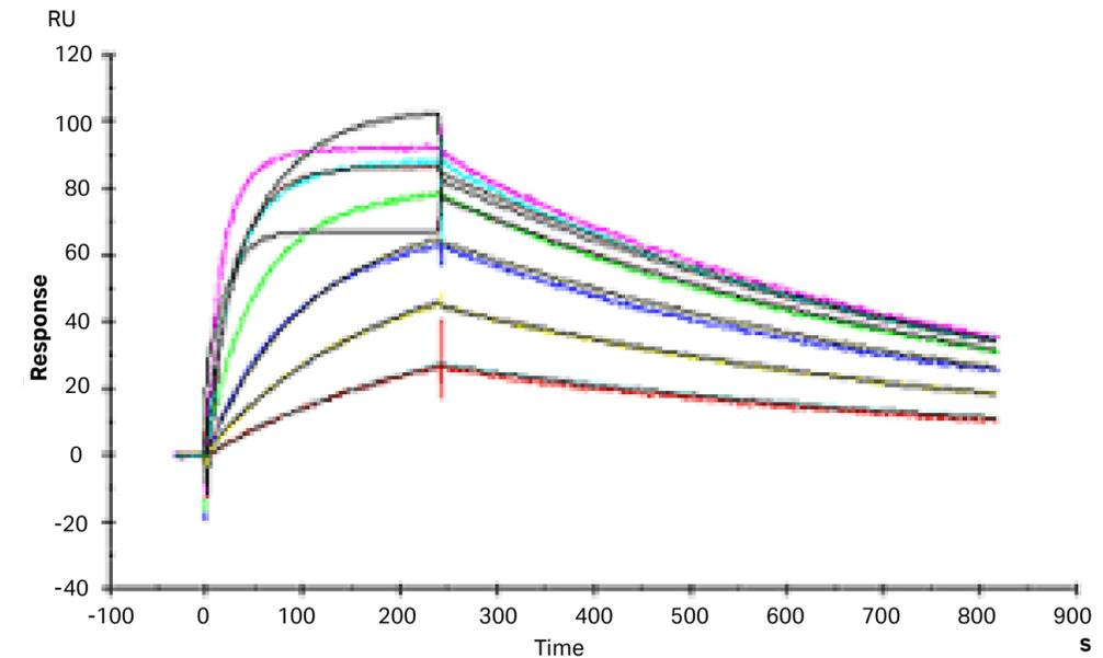
Pipetting error results in two sample concentrations interchanged in the microplate.
