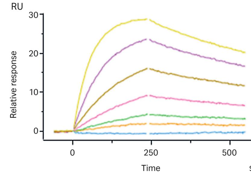
Ideally, the sensorgram for at least one analyte concentration should approach steady state during sample injection.
