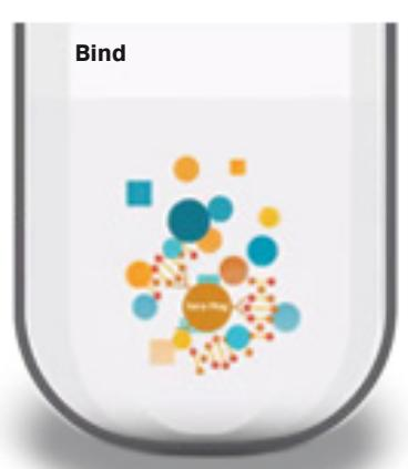
Magnetic particles are captured and remainder of sample is washed away
