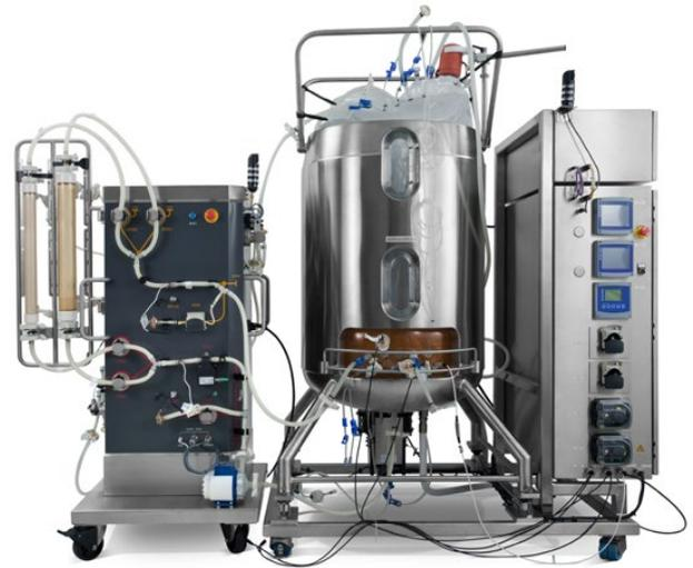
**Fig 6.** Xcellerex™ APS with Xcellerex™ XDR-500 bioreactor.
