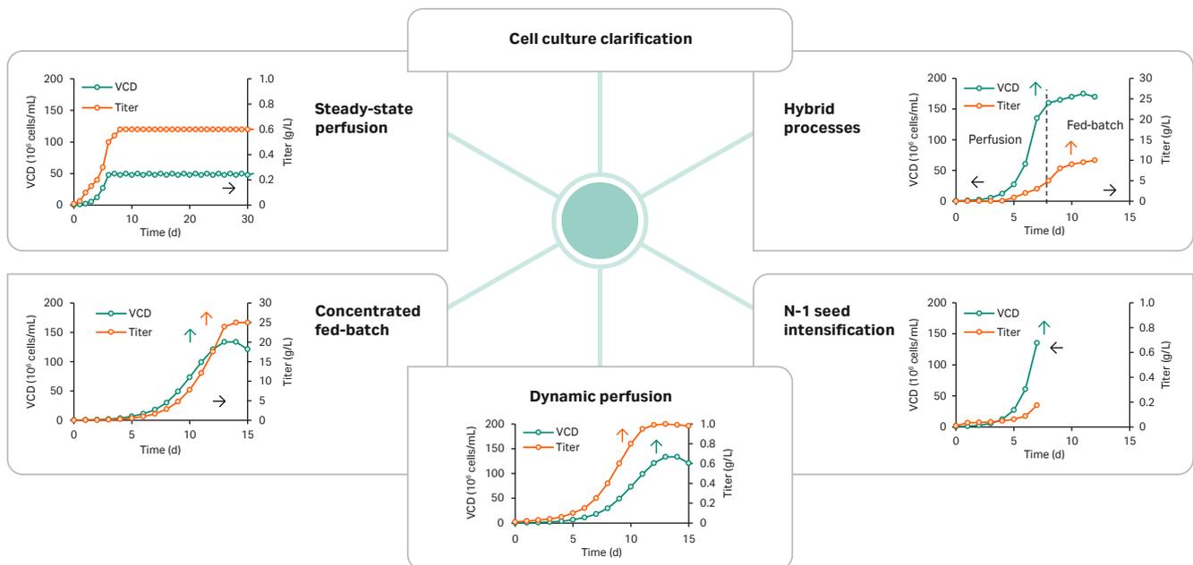
**Fig 7.** Typical perfusion applications for Xcellerex™ APS.
