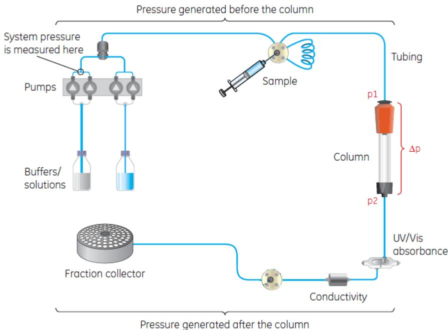
System pressure, generated by the complete system flow path, is measured in ÄKTA chromatography systems at the system pump.  $\Delta p = p_1$  (pressure generated after and by the column itself) –  $p_2$  (pressure generated after the column).
