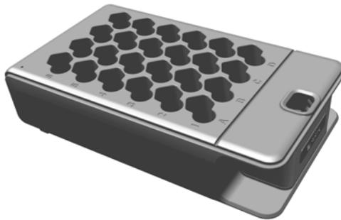
Cooling rack for 1.5 mL and 2 mL tubes. The cooling rack can keep fractions cold for up to three hours. It is prepared by adding water and putting it in a freezer until the water is frozen. The tubes are placed in the rack with their lids bent backward.
