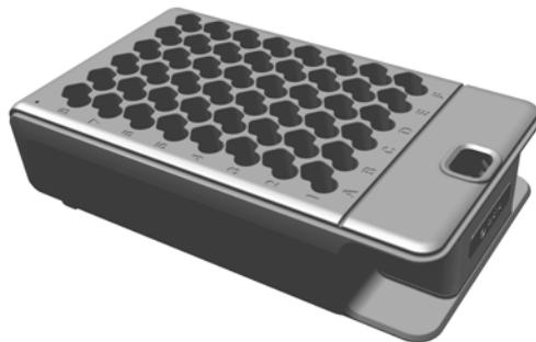
Cooling rack for 0.5 mL tubes. The cooling rack can keep fractions cold for up to three hours. It is prepared by adding water and putting it in a freezer until the water is frozen. The tubes are placed in the rack with their lids bent backward.
