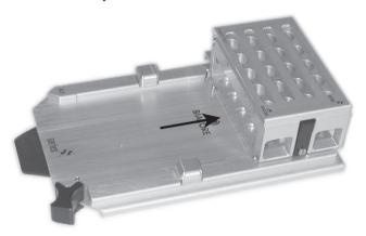
2 Slide the new rack into the holder on the rack tray from the back of the tray. Make sure that it is correctly oriented. The rack can only be fully inserted in one orientation.
