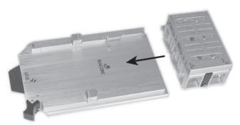
Push the rack until it snaps into position on the rack tray. Make sure that the rack is properly in place.
