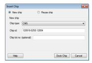
If you are re-using a chip that has previously been docked in the instrument, choose *Reuse chip* and select the *Chip id* from the list. A chip that has been previously used in a different instrument will not be included in the list and must be inserted as a new chip.
