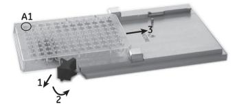
4 Close the catch and make sure that the microplate is properly seated on the rack tray.
