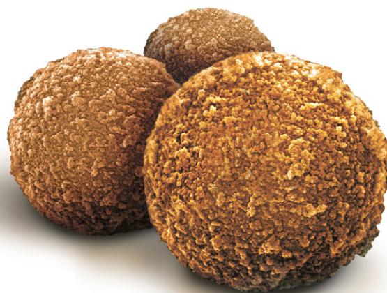
Fig 4. SEM image showing the cauliflower-like surface of the Sera-Mag™ SpeedBeads that dramatically increases the overall surface area available for binding.
