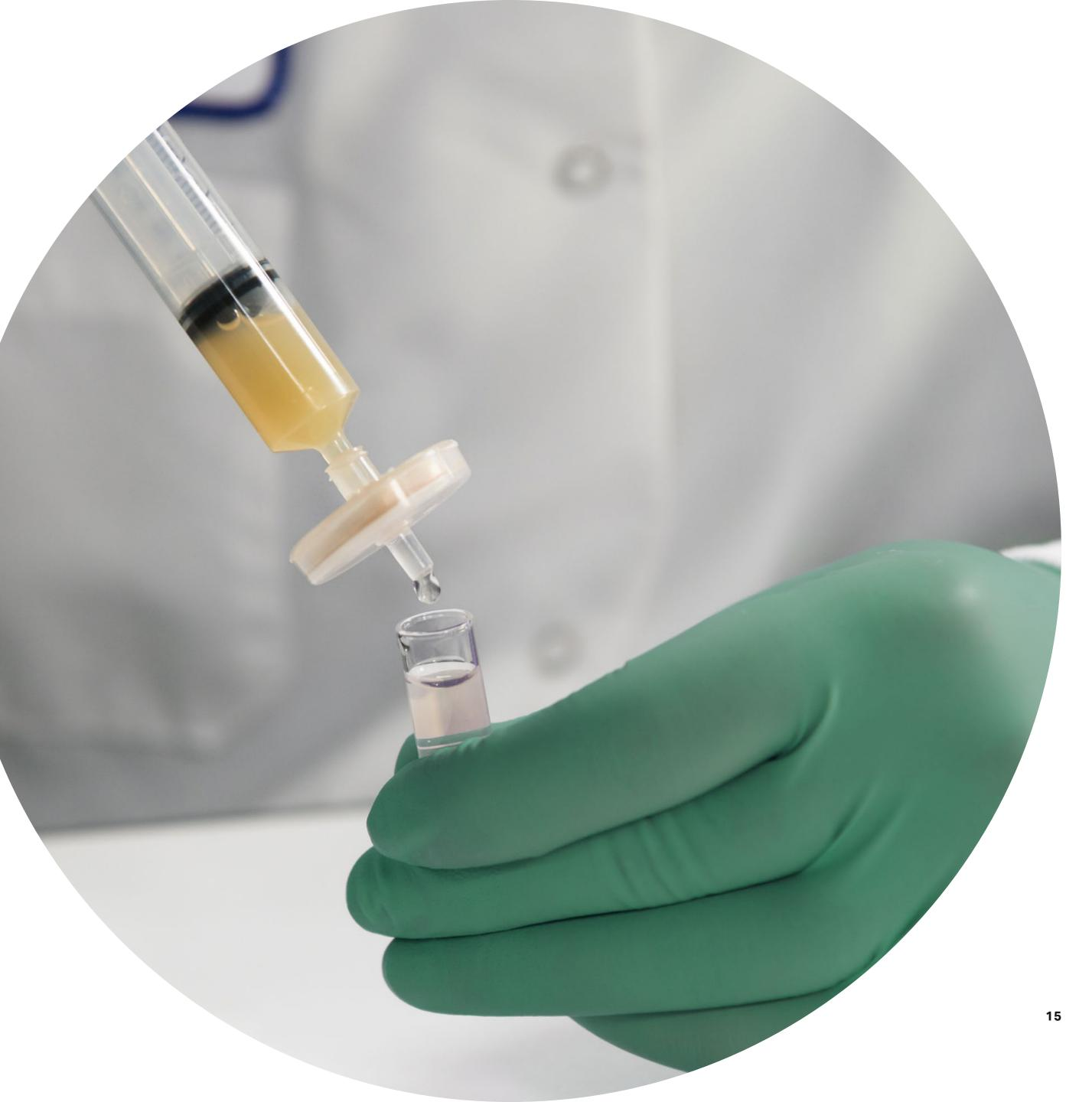
Refers to sterilization by filtration for small sample use which is an industry term for filters of pore size 0.2 µm or smaller as referenced in guidance such as EPA Guidance for Industry Sterile Drug Products Produced by Aseptic Processing — Current Good Manufacturing Practice Section IX, Part B (September 2004).
