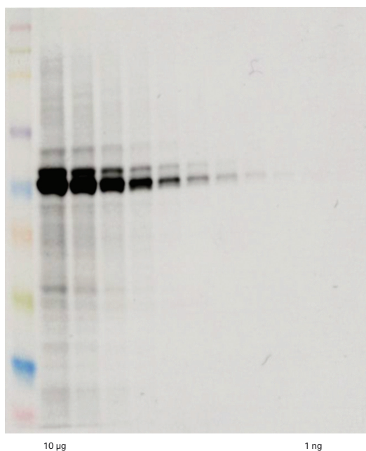
Fig 7. The chemiluminescence mode allows simultaneous imaging of chemiluminescent signals and a colored molecular weight marker. The overlay functionality provides a fast and easy way to verify the molecular weight of detected bands, and identification of band of interest if multiple bands are generated. Amersham ECL™ Prime detection of ERK1/2 in cell lysates from HeLa cells with ImageQuant™ 500.
