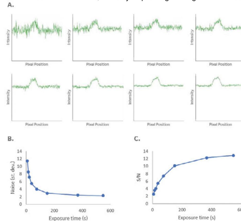
**Fig 8.10.** Image capture and averaging by SNOW algorithm reduces noise to maximize S/N. (A) Line profiles from continuously averaged 7.5 s exposures with SNOW algorithm, from first capture to the average after capture 73, shown by (B) a reduction in noise and stable signal and resulting in (C) an increase in S/N.
