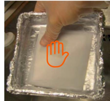
**Fig 10.6.** Do not touch the membrane without gloves - use forceps!
