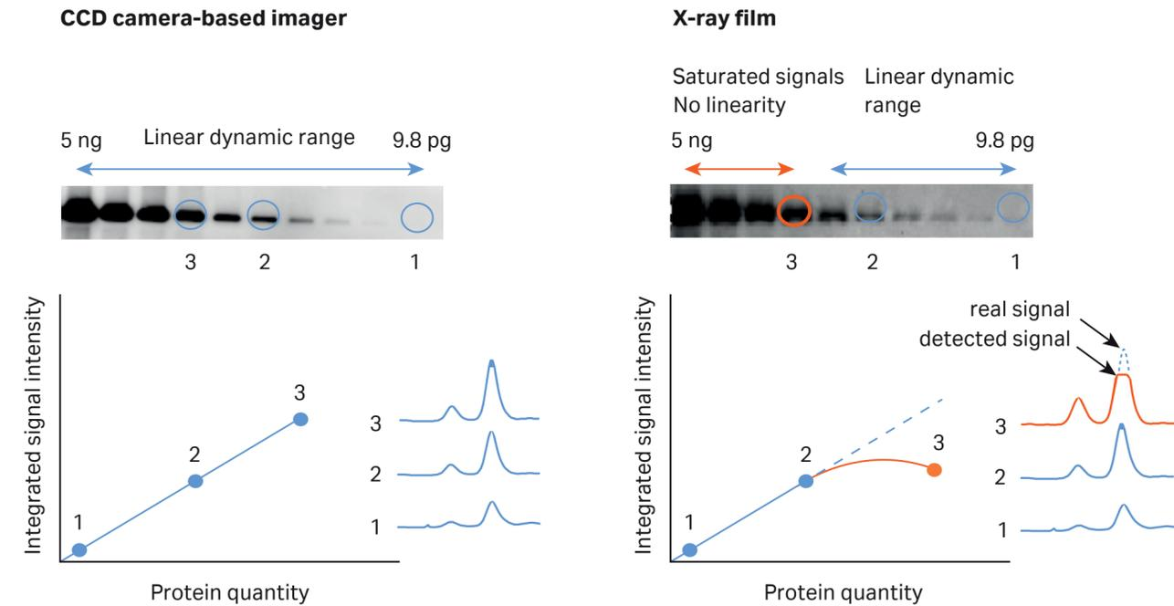
**Fig 8.1.** The advantage of using a CCD camera-based imager compared to X-ray film for signal detection. For the CCD camera-based system, all bands fall within the linear dynamic range of the system, whereas for film, the most intense bands (indicating more protein) are saturated, rendering quantitation impossible at this portion of the curve as the volume under the curve can no longer be determined.
