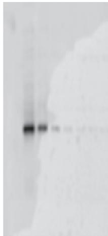
**Fig 10.2.** An insufficiently dried membrane shown with very weak bands on the right.
