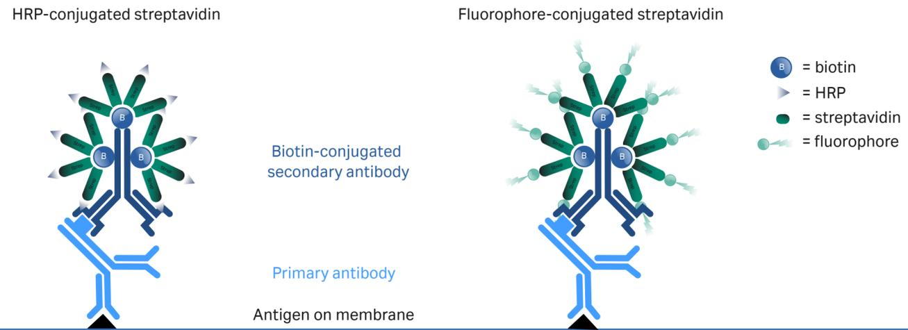
**Fig 9.8.** The principle of three-layer fluorescent Western blotting, where the secondary antibody is labeled with biotin. A third layer of streptavidin conjugated with an enzyme, such as HRP (left) or a fluorophore, such as a CyDye™ (right) as the detection reagent leads to a significant increase in sensitivity compared with two-layer detection.
