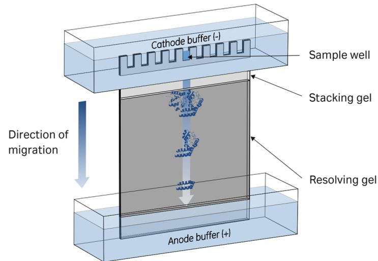
**Fig 3.1.** A vertical electrophoresis apparatus is set up with cathode (-) buffer in an upper chamber and anode (+) buffer in a lower chamber. Molecules in sample wells migrate toward the anode (+) in an electric field. After a set amount of time, the molecules will have migrated to positions based on their size, shape, and charge. As an alternative to vertical electrophoresis systems, horizontal systems are also available.
