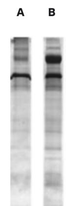
**Fig 2.1.** Comparison of SDS-PAGE Clean-Up Kit with ethanol precipitation. (A) Urinary protein precipitated with 10 volumes of ethanol. (B) Urinary protein precipitated with SDS-PAGE Clean-Up Kit. More and stronger bands are detected after use of SDS-PAGE Clean-Up Kit due to the efficient precipitation procedure the kit is based on. Gel: 8 × 9 cm, 12.5% acrylamide, 0.1% SDS, run on SE 260 Mini-Vertical Unit. Stain: Coomassie Blue R-250.
