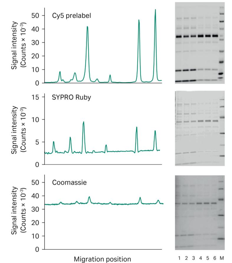
**Fig 3.9.** SDS PAGE analysis of the same protein mixture (300 ng) prelabeled with Cy5 (A) or post-stained with SYPRO Ruby (B) or Coomassie (C). Lane profiles compared after SDS PAGE and imaging show that Cy™5 prelabeling improved sensitivity, and reduced background and noise levels.
