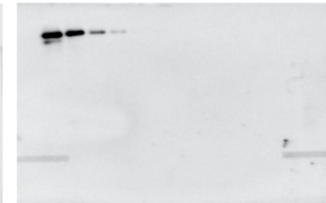
**Fig 4.3.** Comparison of blots following wet and semidry transfer. A two-fold dilution series of transferrin starting at 5 µg was transferred to Amersham Hybond P (now replaced by Amersham Hybond P 0.45) membranes (PVDF). Semidry transfer is less efficient for this particular protein than wet transfer; less protein throughout the dilution series is transferred, leading to reduced sensitivity.
