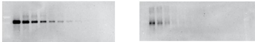
**Fig 10.3.** SDS included in the running buffer (left) gives distinct bands on the membrane. Sensitivity is reduced and protein bands are more diffuse when SDS is absent as seen by the image on the right.
