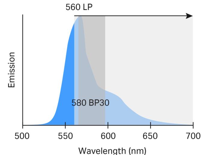
**Fig 7.4.** Emission filtering of Cy<sup>TM</sup>3 fluorescence using either a 580 BP30 filter (dark-gray area) or a 560 LP filter (light- and dark-grey areas). BP = band pass. LP = long pass.
