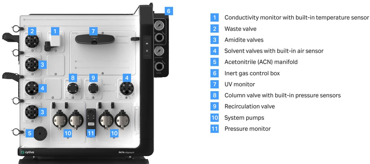
**Fig 3.** System modules for ÄKTA oligosynt™ synthesizer.
