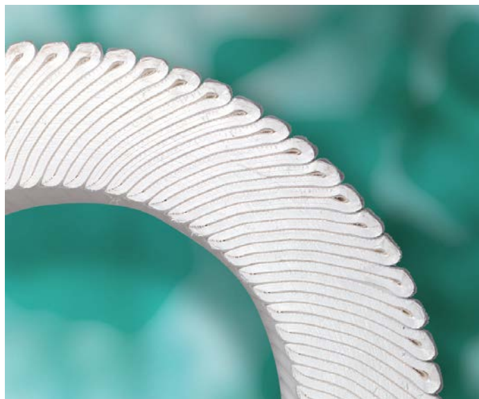
Fig 4. All sizes use 16 layers of Mustang Q membrane in Ultipleat® structure.
