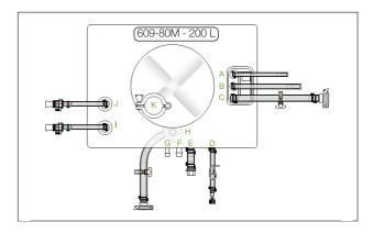
Single-use mixer systems can also be designed according to specific application requirements. Appropriate filters (sterilizing grade/bioburden/mycoplasma reduction) and Kleenpak sterile connectors for sterile fluid addition can be incorporated into system designs. For a customized design, please contact your Pall representative with your specific application details.
