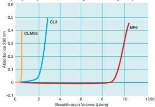
Lysozyme breakthrough curves above demonstrate the high breakthrough capacity of Mustang S capsules. After preconditioning and equilibration with 10mM MES pH 5.5, a solution of 1.6 mg/mL, 2 mg/mL and 1.4 mg/mL of lysozyme in 10mM MES pH 5.5 was pumped respectively through the 10 mL, 60 mL and 260 mL capsules at a flow rate of 10-20 CV/min. The absorbance at 280 nm was continuously monitored downstream of the capsule.
