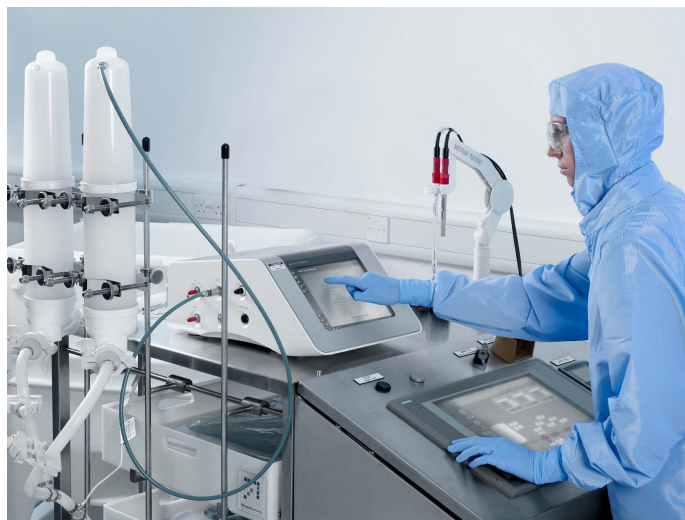
Fig 6. Kleenpak Nova filter capsules undergoing integrity testing.
