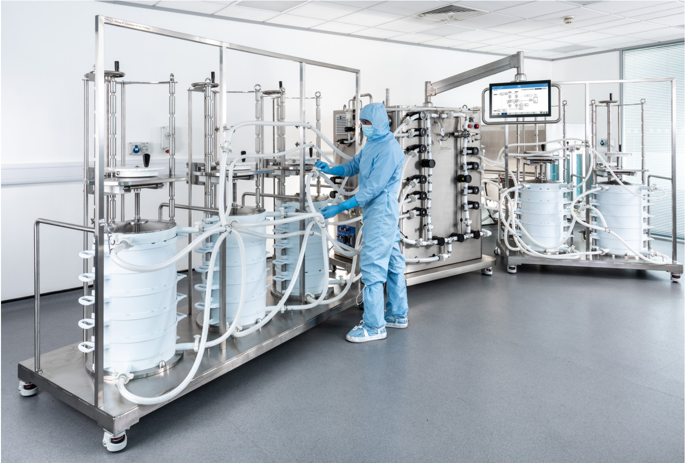
Fig 3. Allegro Connect depth filtration system showing depth filtration stages.
