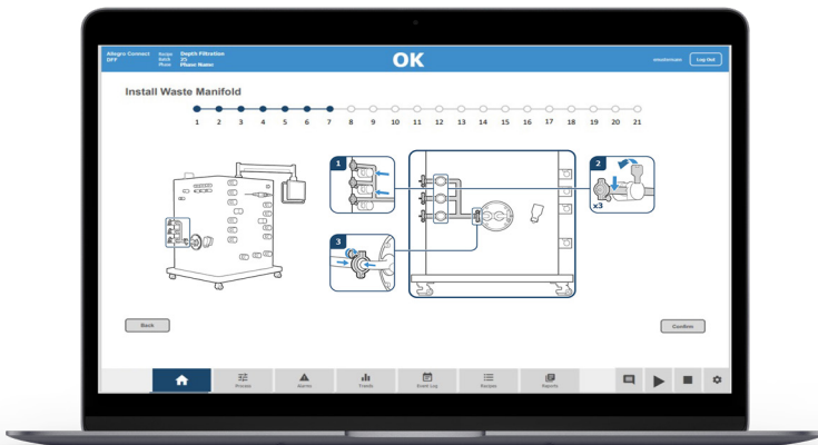
Fig 9. Guided IFI, where the operator is instructed by the recipe to install the waste manifold.
