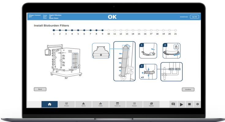
Fig 10. Guided IFI, where the operator is instructed by the recipe to install bioburden filters.
