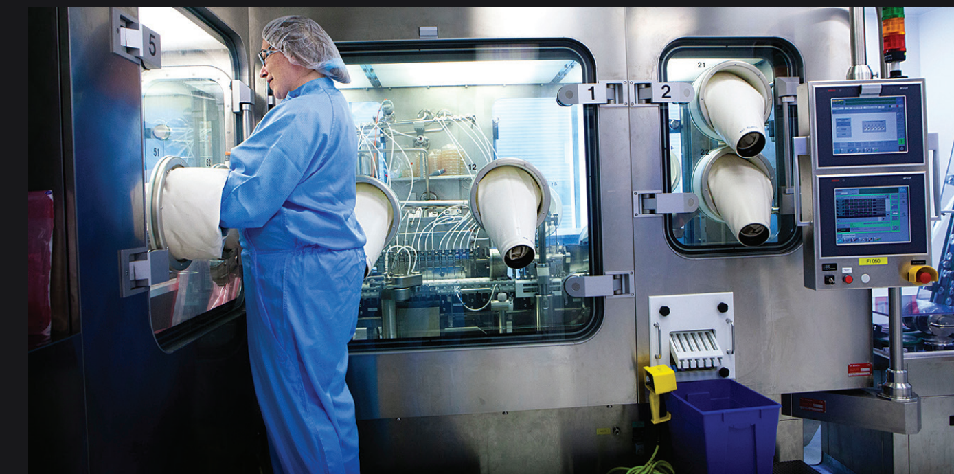
A conventional filling system with glove ports
