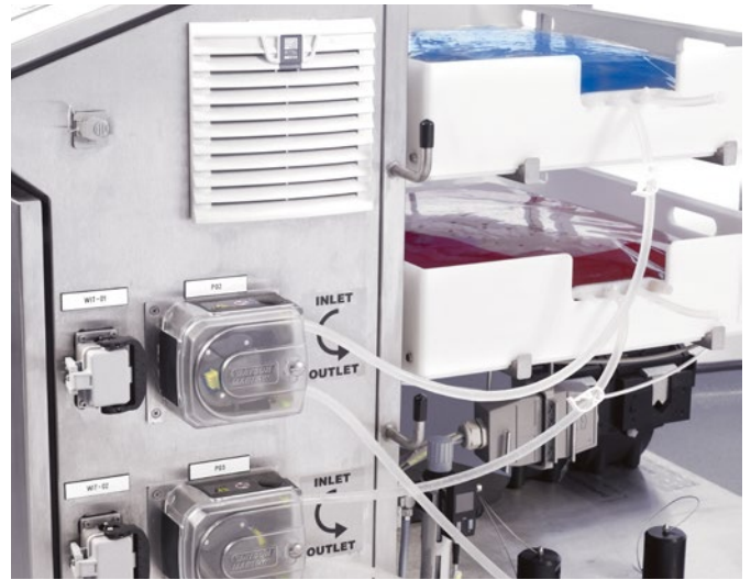
Fig 5. Integral trays containing process fluids.
