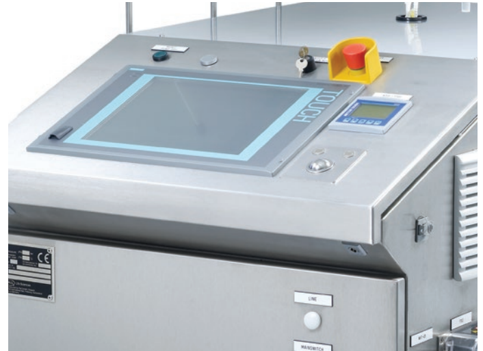
Fig 7. Visual instructions for operators are accessible via the HMI screen.
