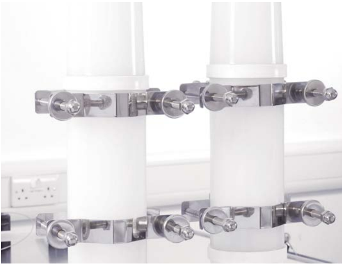
Fig 4. Capsules are supported on the Allegro MVP system with universal clamps.
