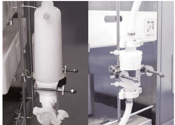
Fig 3. A universal clamp can be used to support capsules with diameter 5 to 10.5 cm.
