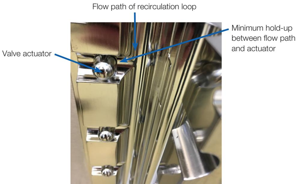
In order to validate these design choices, as well as to demonstrate that the Cadence VI system is free of hold-ups, a series of tests were performed. Riboflavin was used as a visual test for hold-ups and the bacterium *Brevundimonas diminuta* was used to thoroughly scrutinize the system for dead-legs. Finally, experiments were performed with the bacteriophage Phi6, to mimic a mammalian virus.
