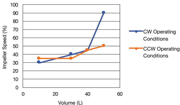
After the maximum usable mixer speed, at which foaming does not occur, was determined the mixing efficiency was assessed for the clockwise and counter clockwise operation at the maximum working volume (50 L) and a lower working volume (10 L). The mixing time was determined using a conductivity probe and measuring the time it took for the conductivity to become stable after an addition of NaCl via the top port of the mixer. The data is shown in Table 2.
