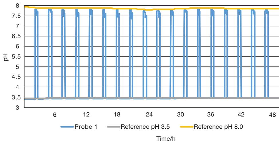
It is apparent from the data that the probes exhibited minimal drift through the course of the experiment. We can look at measurements made at the beginning of the experiment, at the middle of the experiment (at 24 hours) and at the end of the experiment (after 48 hours) and see that the pH probes accuracy remains well within 0.1 pH units, Table 1.
