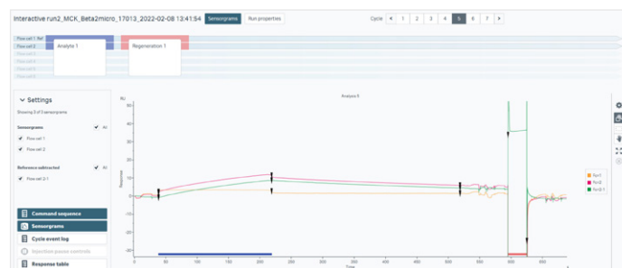
Fig 16. Example of an Interactive run . Each cycle contains an analyte injection (variable concentration) and a regeneration step. The full data set was then fitted to a 1:1 model in Biacore Insight Evaluation Software (data not shown). (Analyte: beta-2-microglobulin. Ligand: Anti-beta-2-microglobulin amine coupled to Sensor Chip CM5).
