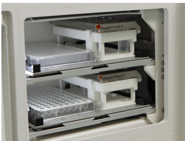
Fig 4. The sample hotel of Biacore 1K+ and Biacore 1S+ accommodates two trays. Each tray can hold one 96-well or 384-well plate and one reagent rack.
