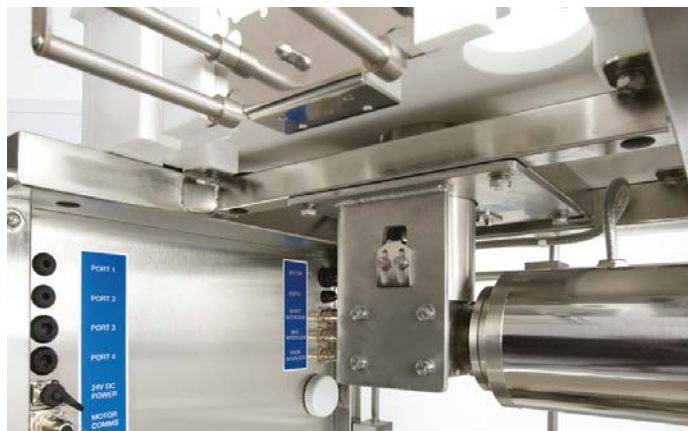
Fig 2. Allegro 50 L mixer motor and UCI.
