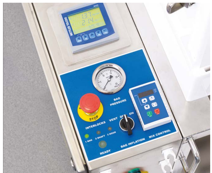
Fig 4. Allegro 50 L mixer user control interface (UCI).
