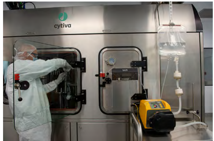
Fig 5. Flowpath installed on the SA25 aseptic filling workcell.
