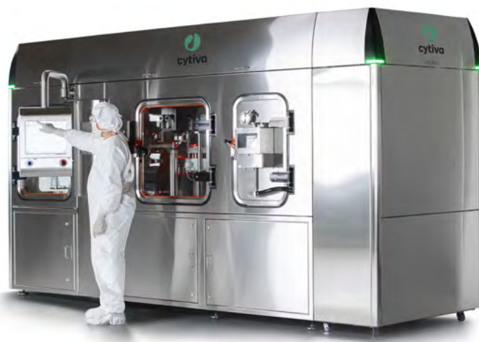
Fig 1. SA25 aseptic filling workcell.
