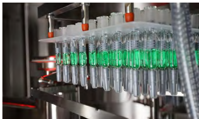
Fig 8. Fully stoppered nested syringes.
