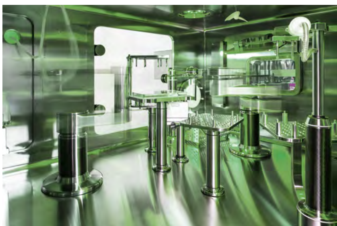
Fig 2. Robotics in motion inside the SA25 aseptic filling workcell.
