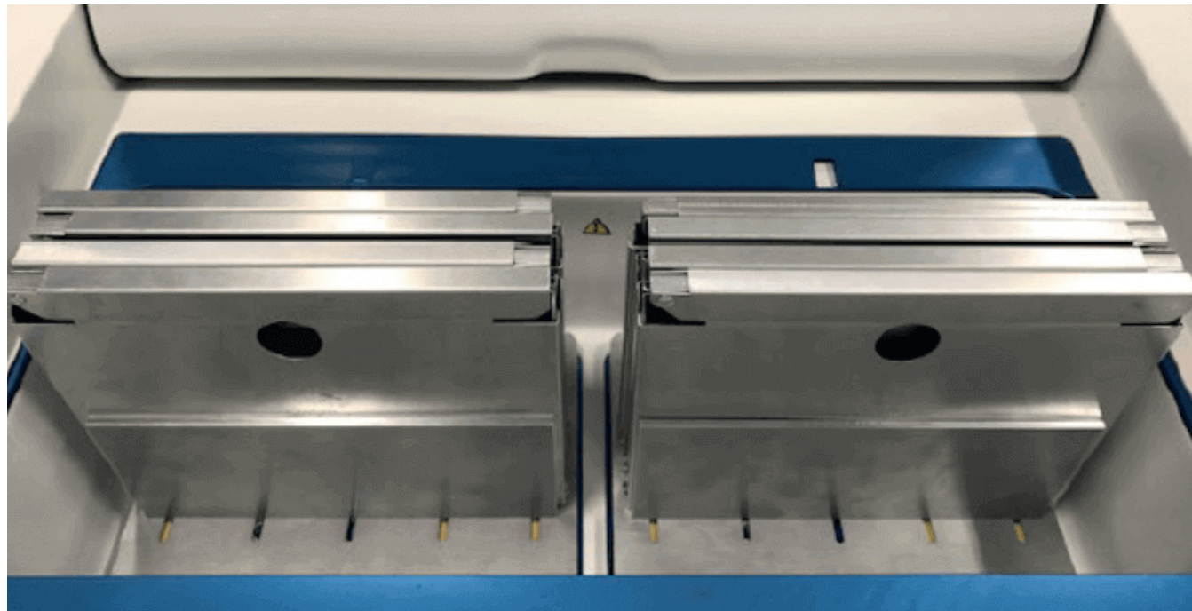
Fig 1. A view of the cryochamber within the VIA Freeze™ Quad unit with sample plates loaded with 8 x 70 mL cryobags held in metal cassettes.
