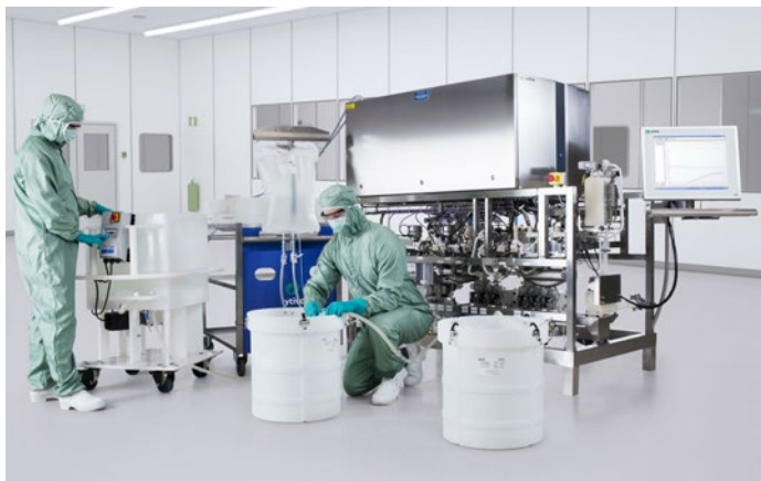
Fig 2. A HyClone single component concentrate solution being used as a source component in the BioProcess IC unit.
