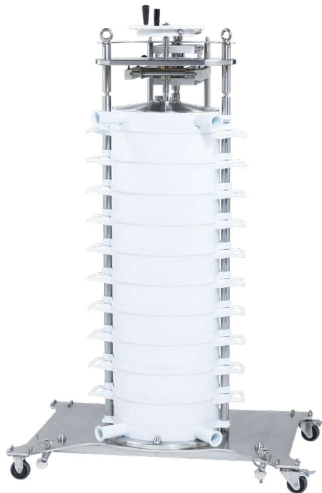
Fig 17. Mount pipe support on 10-high process scale chassis.
