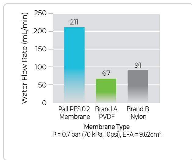
Pall polyethersulfone membrane flow rate outperforms nylon and PVDF membranes of the same pore size (0.2  $\mu\text{m}$ ).
