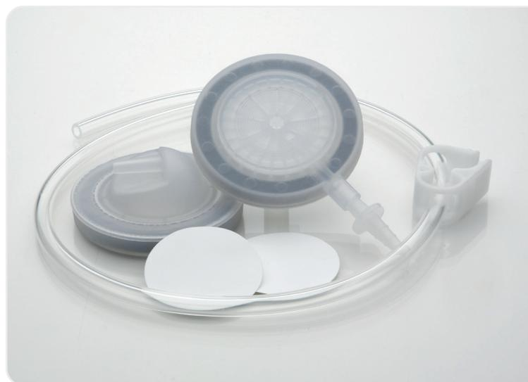
Figure 3: The SolVac filter holder
