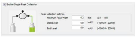
Single Peak Collection option is available when Frac30 has been disabled from the instrument. Single Peak Collection can be chosen and configured in the *Elution and Fractionation* phase as depicted above.
