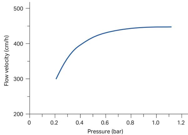
**Fig 2.** Pressure/flow curve for Butyl Sepharose 4 Fast Flow in an XK 50/30 column, bed height 150 mm, mobile phase 0.1 M NaCl (work from Cytiva).
