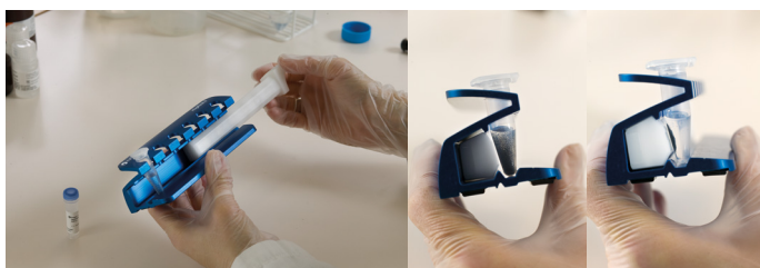
Fig 2. The high density of the beads allows rapid capture by MagRack 6 magnetic device.
