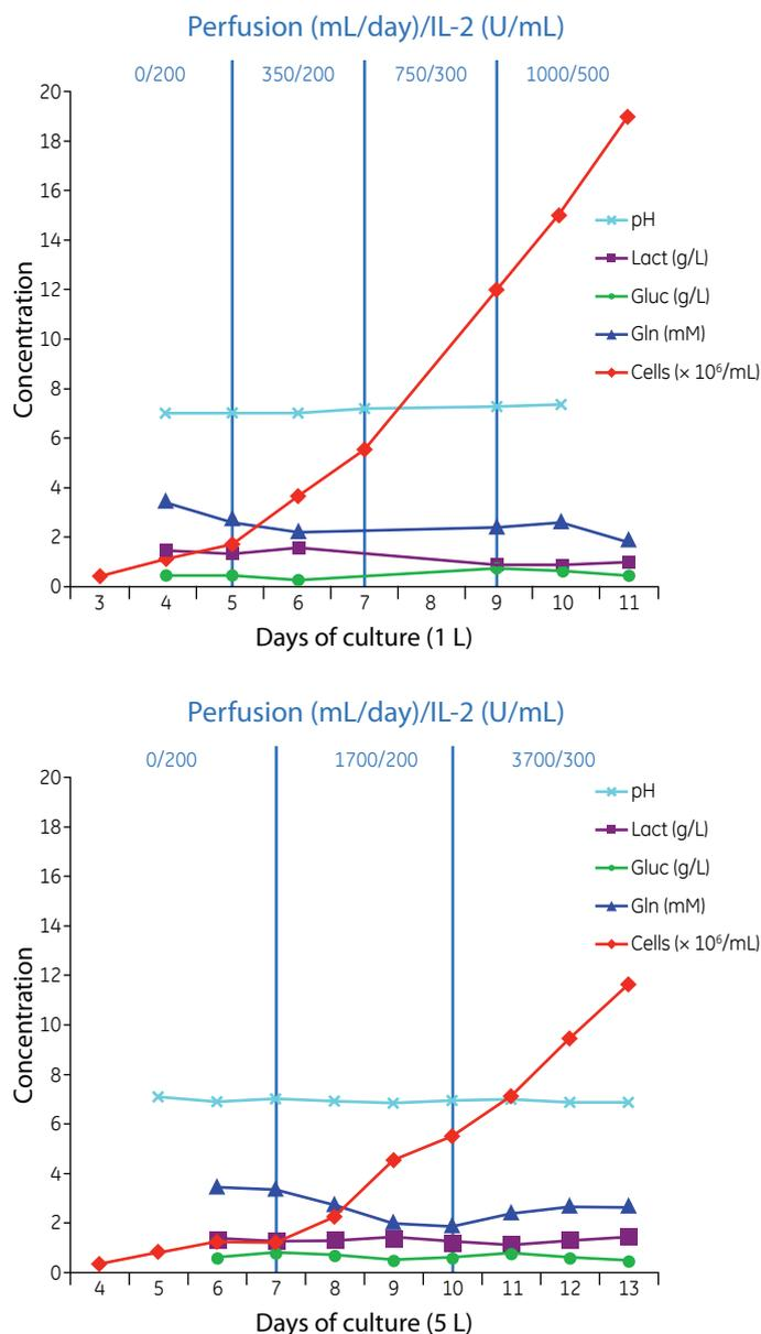
**Fig 3.** Cell density gradually increases during expansion in the WAVE Bioreactor System 2/10 whereas pH and levels of metabolites and nutrients are kept constant by increasing the perfusion rate. Data from one 1 L culture (with increasing rocking) (top) and the 5 L culture (bottom) are shown.
