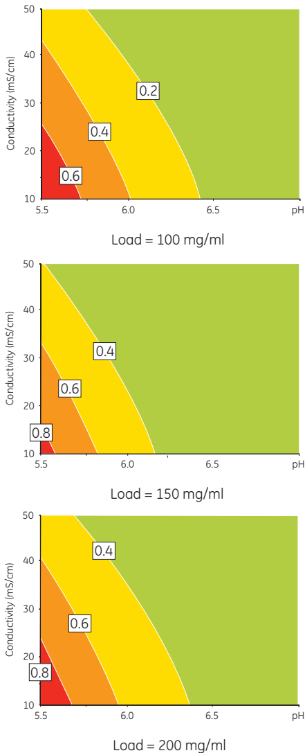
Fig 4. Response surface plots demonstrating the effect of pH, conductivity, and load on the clearance of aggregates. High pH, high conductivity, and low load gives the best reduction of aggregates. Aggregate concentration in the flowthrough pool is expressed in percent (labels).
