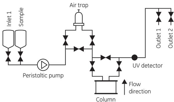
Fig 2. Schematic drawing of the system configuration.
