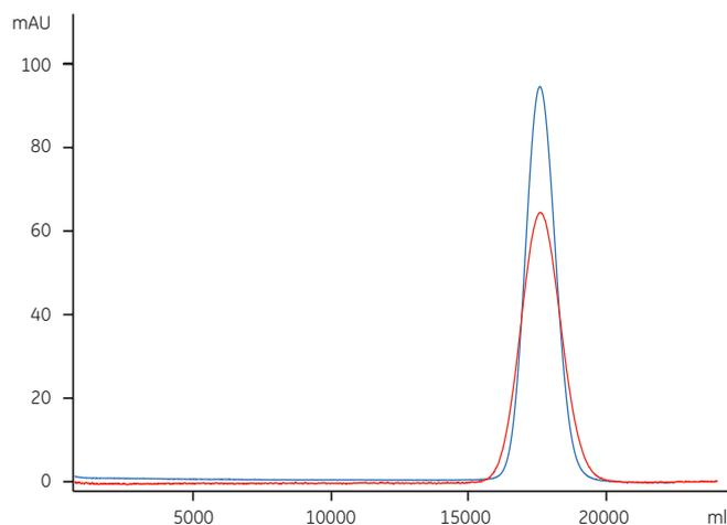
**Fig 5.** Sample peak with a liquid velocity of 30 cm/h (blue curve) and 100 cm/h (red curve).
