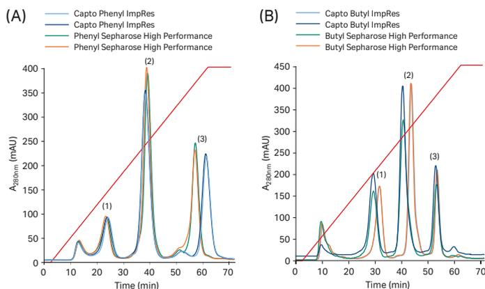
**Fig 4.** Selectivity test using three model proteins, ribonuclease A (1), lysozyme (2), and  $\alpha$ -chymotrypsinogen (3). (A) Comparison of Capto Phenyl ImpRes with Phenyl Sepharose High Performance. (B) Comparison of Capto Butyl ImpRes with Butyl Sepharose High Performance.
