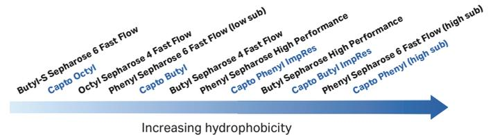
**Fig 3.** Relative hydrophobicity of HIC media. Products marked in blue are based on high-flow agarose (Capto) for increased productivity.
