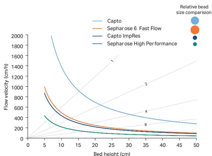
**Fig 5.** The window of operation (area under the curve) of different media from Cytiva. Data correspond to a 1 m diameter column at 20°C and viscosity equivalent to water. Gray contours show the residence time in the column in minutes.
