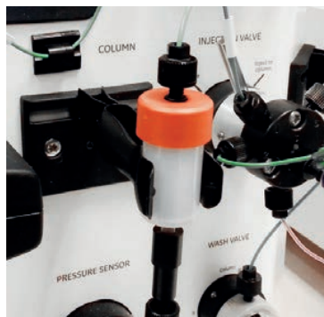
Fig 5. Image showing the column position.
