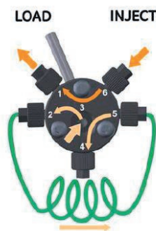
Fig 6. Image showing Manual injection valve in LOAD position and sample loop attached to ports 2 and 5.
