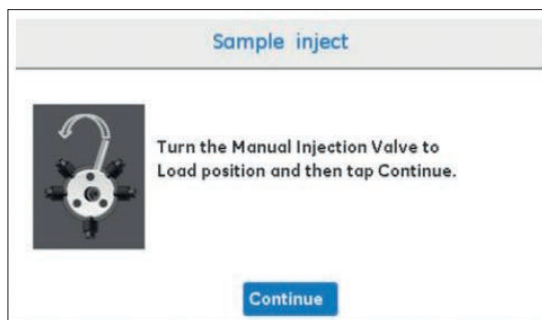
Fig 13. ÄKTA start display: Screenshot of Sample inject message screen prompt following sample injection.
