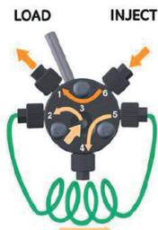
Fig 5. Image showing Manual injection valve in **LOAD** position and sample loop attached to ports 2 and 5.
