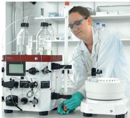
Fig 4. Image showing the gel filtration column being attached to the AKTA start instrument.
