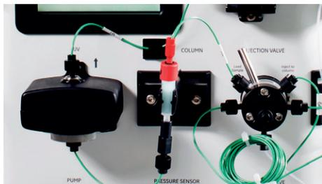
Fig 7. Image showing the column position.
