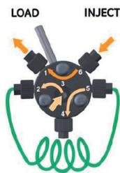
Fig 8. Image showing Manual injection valve in **LOAD** position.
