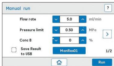
Fig 4. ÄKTA start display: Screenshot of the **Manual run** screen (1/2).
