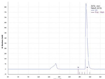
Fig 14. Chromatogram (.bmp image) of affinity purification on ÄKTA start.
