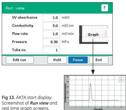
Fig 13. ÄKTA start display: Screenshot of **Run view** and real time graph screens.
