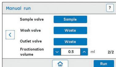
Fig 5. ÄKTA start display: Screenshot of the **Manual run** screen (2/2).
