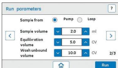
Fig 11. ÄKTA start display: Screenshot of **Run parameters** screen (2/3).
