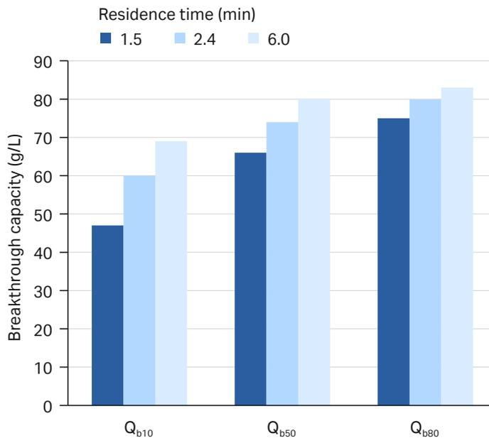
**Fig 7.** Results from breakthrough capacity experiments performed using MAb-containing cell culture feed. Note that capacity increases with increasing residence time, regardless of the breakthrough level. The effect of residence time is strongest at lower levels of breakthrough (e.g.,  $Q_{b10}$ ).
