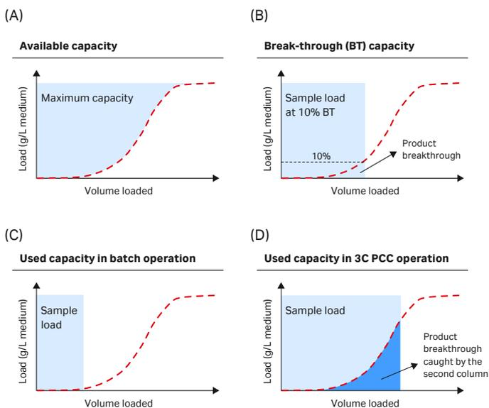
**Fig 6.** Capacity utilization for standard vs PCC. (A) Total available capacity of a chromatography medium. (B) The capacity typically measured during process development experiments. (C) The capacity typically utilized in manufacturing after adding safety factors. (D) Typical capacity utilized when implementing PCC. Note that product breakthrough is captured by the next column in the loading zone.
