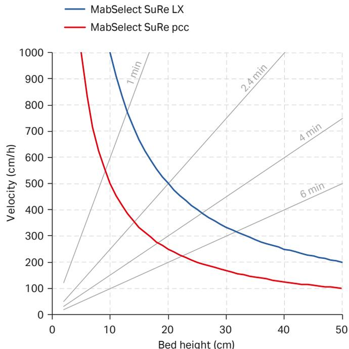
**Fig 3.** Window of operation for MabSelect SuRe pcc versus MabSelect SuRe LX. Pressure limits are assumed to be 3 bar. At 2.4 min residence time, for example, MabSelect SuRe pcc can be packed in beds up to 14 cm in height, whereas MabSelect SuRe LX can be packed at 20 cm bed height.
