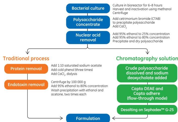
**Fig 1.** Traditional versus proposed meningococcal polysaccharide purification process.
