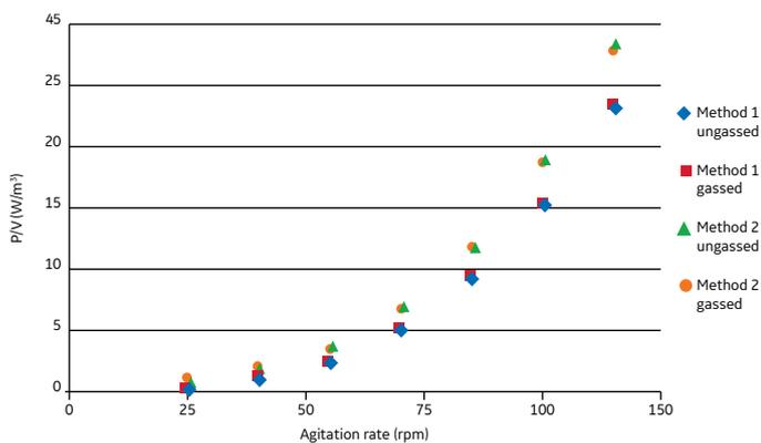
**Fig 6.** Power input per liquid volume ( $P/V$ ) plotted against agitation rate at max. working volume (2000 L) for Method 1 (motor current) and Method 2 (torque sensor) at gassed and ungassed conditions. The air flow was 20 L/min for gassed conditions. Each data point shows the mean value of duplicate runs.
