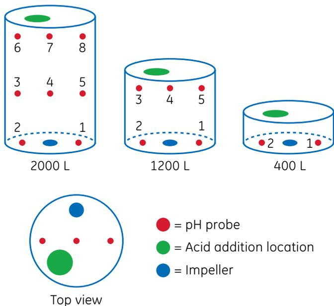
**Fig 2.** The pH probe positions for the tested volumes. Eight probes in three levels were used to record the pH for 2000 L. At 1200 L, the top probe layer was removed and the pH was recorded by using five probes in two levels. At 400 L, the pH probes of the midsection were removed, leaving the bottom pH probes. Acid and base were added from the top as close to the center as possible for all experiments.
