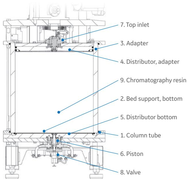
Fig 8. Sanitization of AxiChrom columns. 53 sites were sampled on an AxiChrom 600. The column was packed with Sepharose™ Fast Flow resin and challenged with *E. coli* ATCC 8739 ( $10^6$  viable organisms/mL). There were no surviving *E. coli* after sanitization with 1.0 M NaOH for 5 h. The endotoxin concentration was less than 0.25 EU/mL (USP recommendation for WFI).
