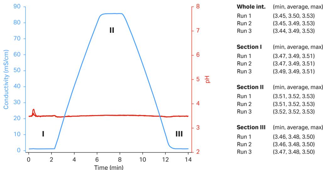
**Fig 2.** Overlay of three chromatograms from preparation of 20 mM citrate buffer, pH 3.5 with an increasing gradient of salt: 0 to 1 M NaCl at 400 L/h (flow feedback control). For this specific run, the accuracy was 0.1 pH units and the robustness 0.02 pH units.
